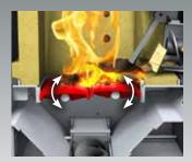
Furthermore, the grates are able to level the firebed to ensure a homogeneous combustion process.
