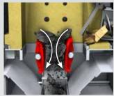
For miscanthus, corn cobs, etc the "Breaker Function" of the grate forces clinker down into the ash auger.
