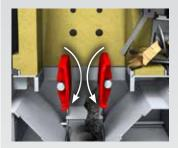
If the boiler is completely cold, a full cleaning process is executed. Both grates rotate and all foreign objects like stones, nails, etc. are removed in addition to the cold ash
