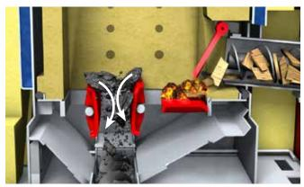
For **miscanthus**, or materials which tend to slag, the added "**breaker function**" forces the ash into the ash box.
