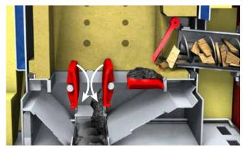
If the boiler is completely cold, a full cleaning process is executed. **Both grates rotate**, so all foreign objects like stones, nails, etc. are removed, as well as the cold ash.
